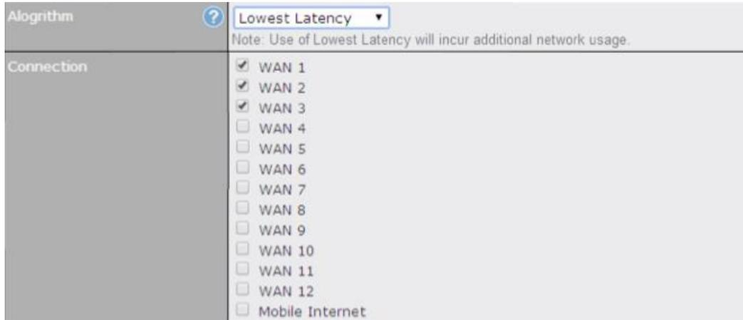
The traffic matching this rule will be routed through the healthy WAN connection that is selected in **Connection** and has the lowest latency. Latency checking packets are issued periodically to a nearby router of each WAN connection to determine its latency value. The latency of a WAN is the packet round trip time of the WAN connection. Additional network usage may be incurred as a result.
