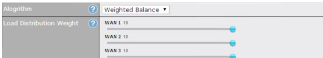
The amount of matching traffic that is distributed to a WAN connection is proportional to the weight of the WAN connection relative to the total weight. Use the sliders to change each WAN's weight.
