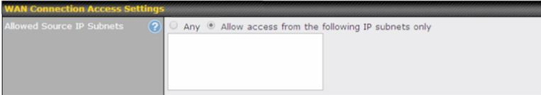
Enter your allowed IP subnet addresses into this text area. Each IP subnet must be in the form of *w.x.y.z/m*. *w.x.y.z* represents an IP address (e.g., *192.168.0.0*), and *m* represents the subnet mask in CIDR format, which is between 0 and 32 inclusively. For example: *192.168.0.0/24*.
