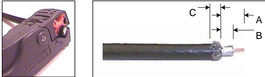
Figure 16: Cutting Technique for Removing Foil in the Braid
