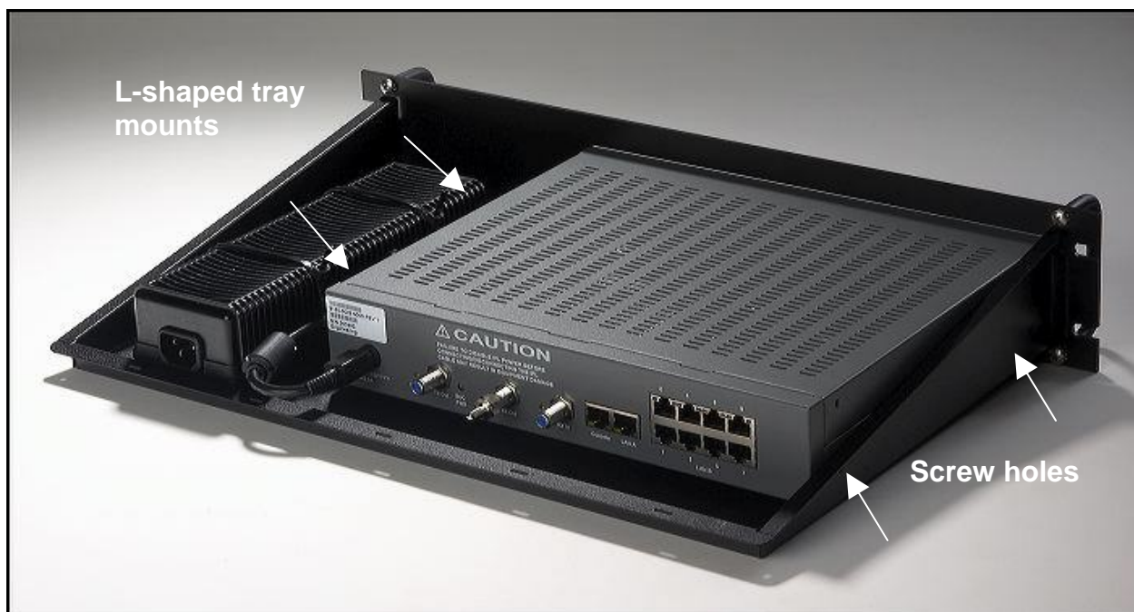
Figure 10: Rear View of an iDirect 5000 series™ Satellite Router in a Rack-Mount Tray
