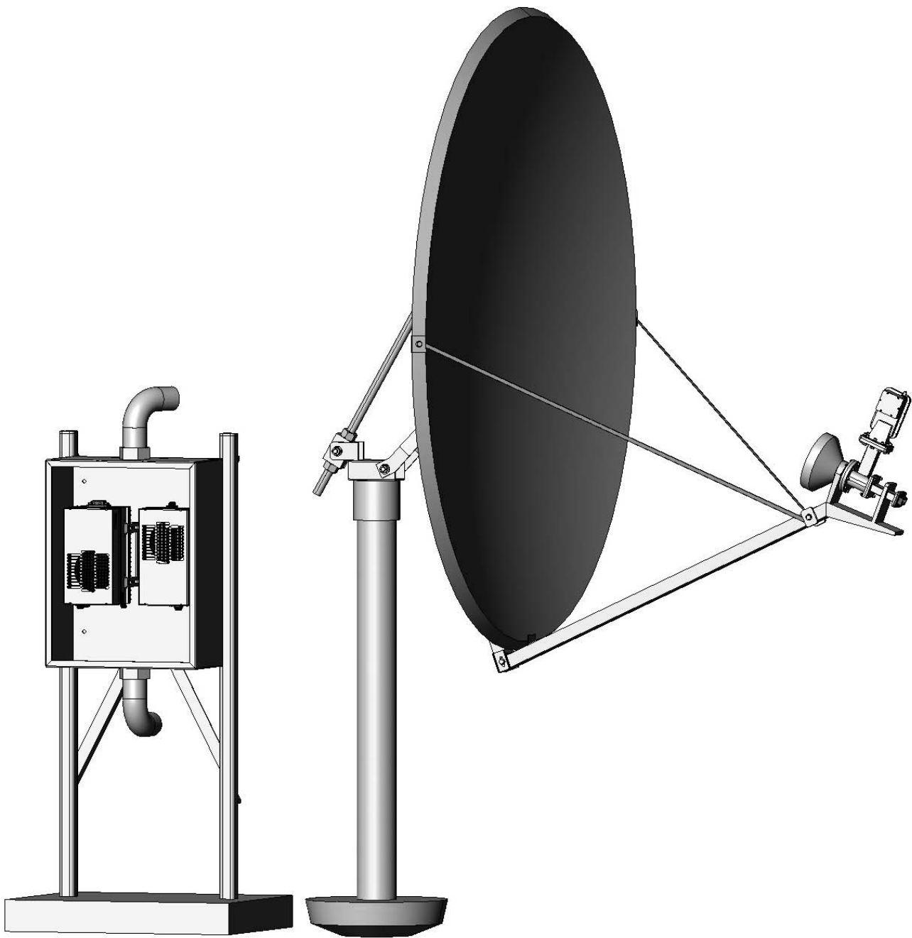
Figure 3.5 Mounting on Antenna Back Structure
